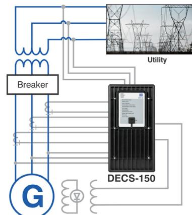
Figure 1 - DECS-150 Connection Diagram for a Typical Application
